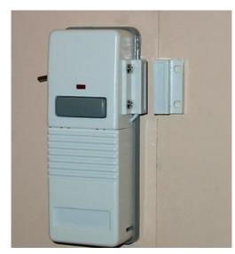
The Sensor Unit is mounted at the top of the door.
